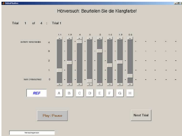
Figure 2-2: Screenshot of the MUSHRA-like interface of the experiment. The software was programmed in MATLAB.
